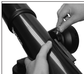
Fig. 7: Attach Vixen-style dovetail to mounting arm.
