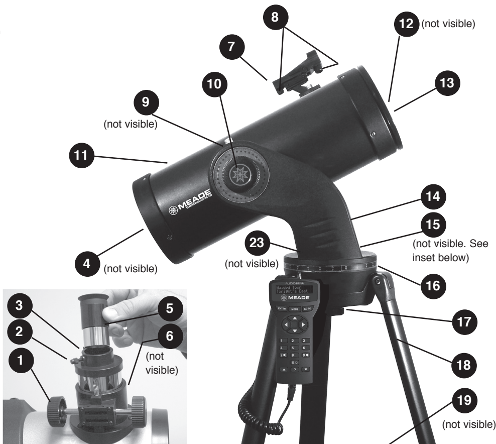
Fig. 2f (Inset): Focuser Assembly.
