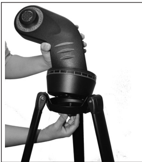
Fig. 6: Attach the mounting arm to the tripod base.
