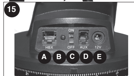
Fig. 2c (Inset): Computer Control Panel. (A) Handbox port; (B) Power indicator light, (C) ON switch; (D) Auxiliary port; (E) 12v Power.
